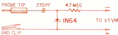
Fig. 7—Rf probe for vtvm. Build the whole thing into some kind of tubular shield.
