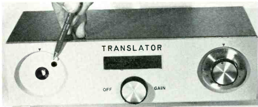
Vhf fine-tuning slugs for each channel are accessible through this hole behind vhf channel-selector knob.
