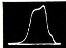
Fig. 13—You must use a demodulator probe to check bandpass frequency response.
